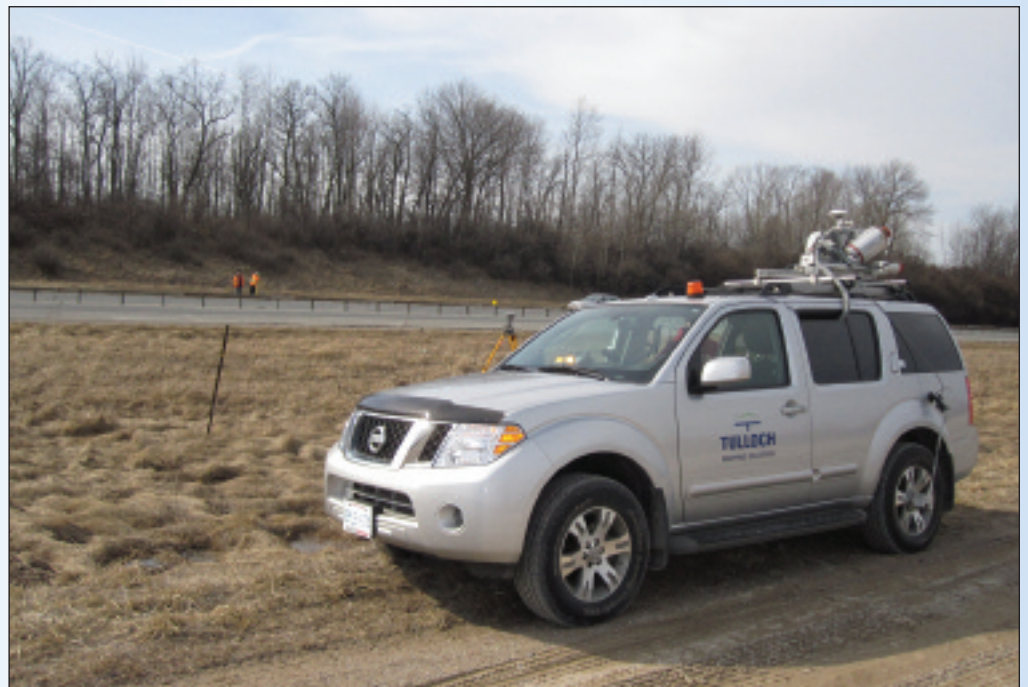
The vehicle mounted MLS system
